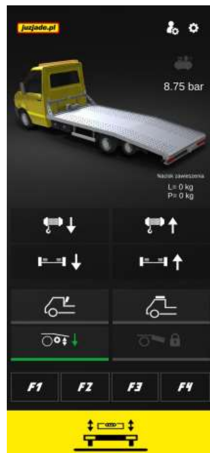
SELF-LEVELING FOR DRIVING WITH THE TRAILER DOWN, ENABLED. THE APP INDICATES THE PRESSURE ON THE TRAILER IN KILOGRAMS (IT AIMS FOR 750 KG)
