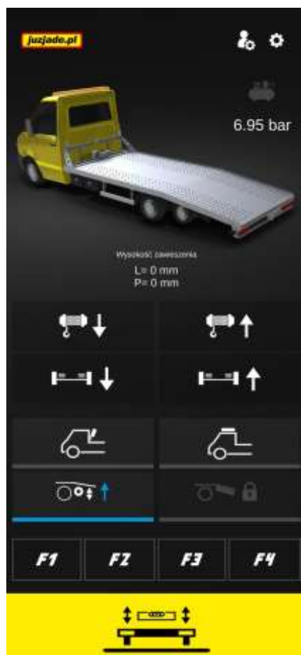
SELF-LEVELING FOR DRIVING WITH THE TRAILER RAISED, ACTIVATED. THE APP INDICATES A REFERENCE LEVEL TO 0 IN MILLIMETERS (AIMS FOR 0 MM)
